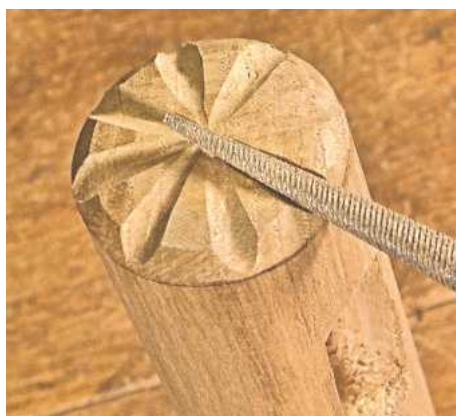
▲ Pic. 3 This time he used a round file to try a bolder decoration
